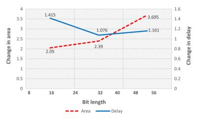
Fig. 16 Percentage change in area and delay with change in word length of various floating-point units in the proposed run-time-reconfigurable multi-precision floating-point multiplier
