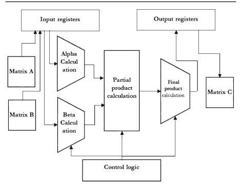
Fig. 3 Block diagram of processing element
