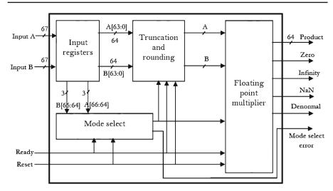
Fig. 4 Block diagram of run-time-reconfigurable variable-precision floating-point multiplier
