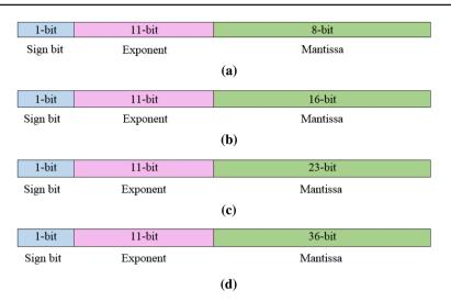
**Fig.6** Custom precision floating-point formats used in the model. **a** Custom precision format 8-bit mantissa, **b** custom precision format 16-bit mantissa, **c** single-precision format, **d** custom precision format 32-bit mantissa
