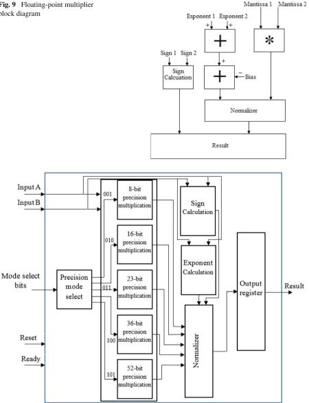
Fig. 10 Block diagram of floating-point multiplier model in the proposed design
